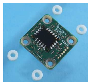
Fig. 8 Four plastic spacers (plastic distance rings) of 1.6 mm thickness are optionally (Table 6) delivered with each encoder in order to mount the encoder on a flat surface and avoid that the components on the backside touch the mounting-surface. The height of the components is 1.45 mm maximum (Fig. 7).
