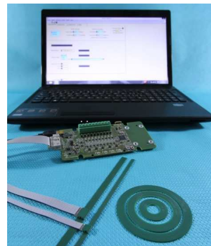
Fig. 4: The Interface Board operated with PC
