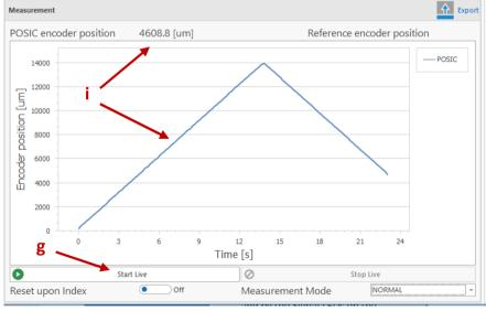
Detailed information about measurements with a reference encoder, linearization, debug and troubleshooting can be found in the ASSIST User Manual, which can be downloaded from POSIC's website.
