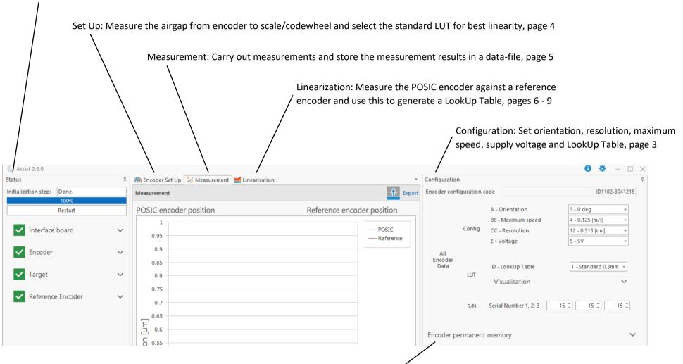
Status: Check Interface Board and Encoder and define target (scale or codewheel) and reference encoder , page 3
