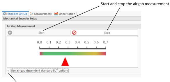
Activate this option: ASSIST automatically selects and loads the best available standard LUT after completion of the airgap measurement.
