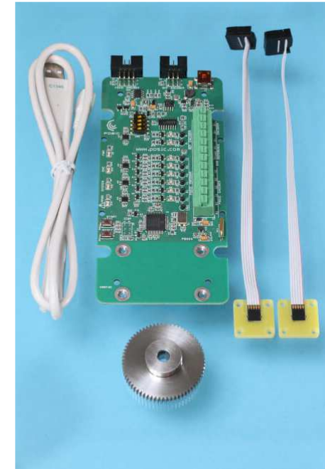
EPT002-ID1102G-0-0 EPT with speed sensors and gear
